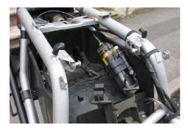
The Dispenser Assembly, shown bottom left, is routed along the underside of the Swingarm using Dispenser Mounting Sleeves & Glue. **Note:** an epoxy resin (eg. Araldite) is reg'd to bond the sleeves to the Swingarm.
